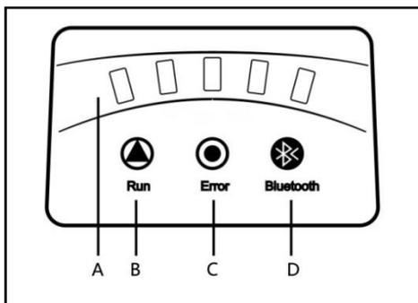
**A: Display board of electrical quantity.** Normally, all five lights will keep brightening when the power is sufficient. Five lights means **Robstep** is fully charged, four means there is 60 % ~80% power left.
